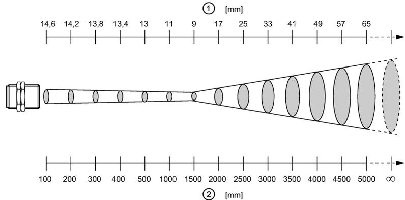
1: diameter of the measured spot; 2: measuring distance
