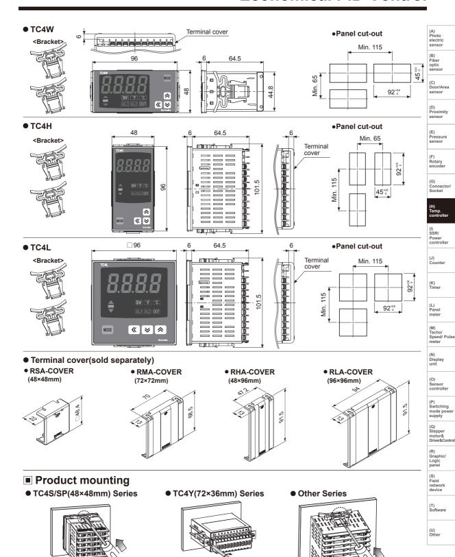
\*Mount the product on the panel, fasten bracket by pushing with tools as shown above. (In case of TC4Y, fasten bolts for bracket.)
