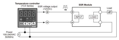
When selecting phase or cycle control mode, the power supply for load and temperature controller must be the same.
