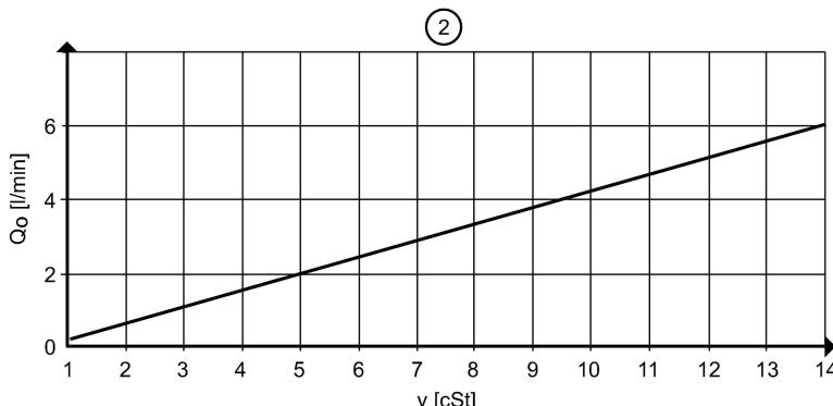
Response threshold  $Q_{\min}$  [l/min] depending on the kinematic viscosity
