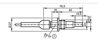
1: tightening torque max. 30 Nm
