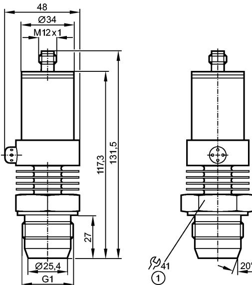
1: tightening torque 20 Nm
