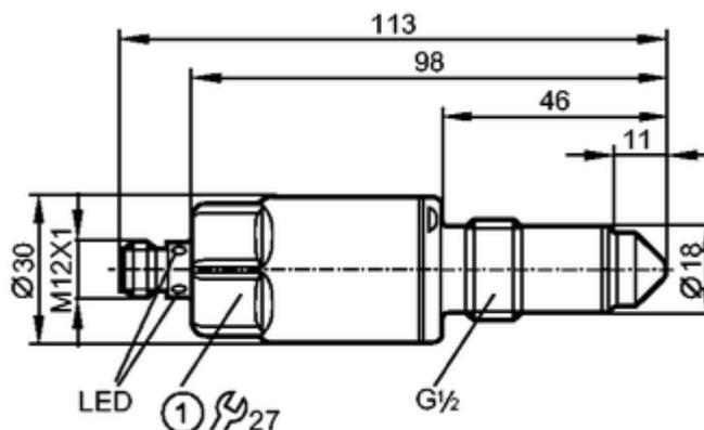
1: tightening torque 20...25 Nm
