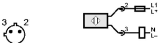
Note: miniature fuse to IEC60127-2 sheet 1, ≤ 2 A (fast acting)
