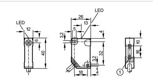
1: threaded insert M3, depth 5.8 mm, max. tightening torque 1.2 Nm (screw fixing class 8.8) when brass insert in contact with counterpart.
